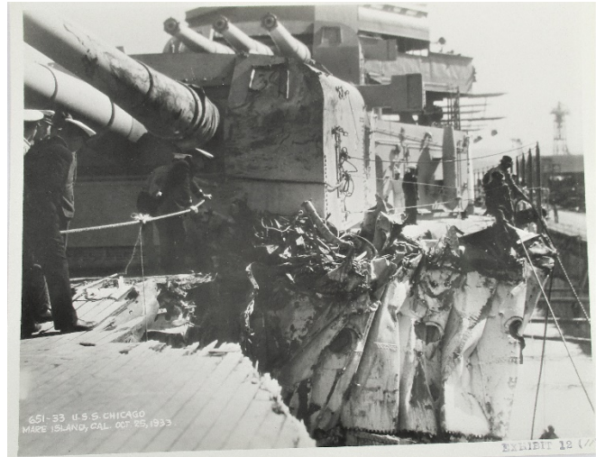
Chicago's damage, portside forward. Photo taken after she was docked for repairs. The accordion-like compression of the hull plating is clearly visible on the aft side of the gash made by Silverpalm. Source: NARA.
