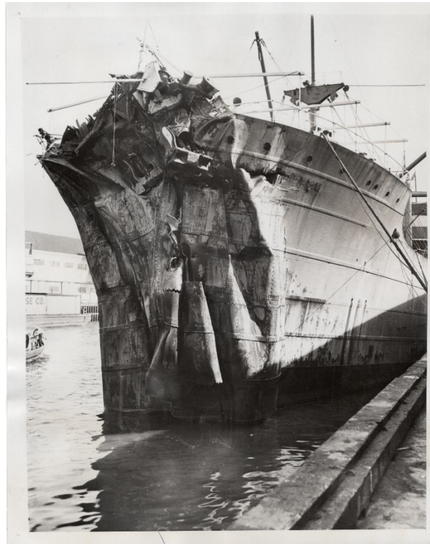
The damaged bow of Silverpalm when the ship docked at San Francisco after the collision.
