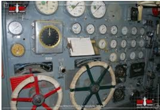
Throttle board of battleship Missouri (BB-63) on the left. The wheel with red spokes controls steam to the turbines when the ship goes astern. The wheel with green spokes controls steam to the turbines when the ship goes ahead. Note the throttlemans log on the clipboard. On the right are the engine revolution counter and engine order telegraph indicator from destroyer The Sullivans (DD-537). There is motion picture film on You Tube of a throttlemans actually changing his throttle and marking his log on destroyer escort Charles E. Brannon (DE-446).
